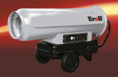
Oil heaters without flue gas pipe. They are suitable for outdoor use or in well-ventilated rooms and have a degree of efficiency of 100 %. Fuel supply from the integrated tank via an integrated compressor with the models "GK". With the models "GP" via an integrated high-pressure pump.
