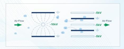
The above diagram shows, in a basic visual, how an electrostatic precipitator works:
