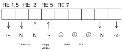
Transmisson:between  $\sim$  and N is always 230V when the transformer handle is in pos. 1-5
