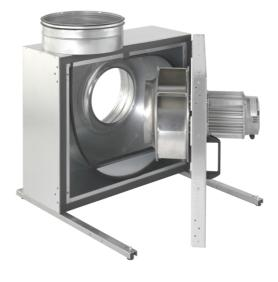
10V for an external potentiometer or sensor. The KBR-EC fans have impellers manufactured from galvanized sheet steel with backward-curved blades. The casing is manufactured from double-skinned galvanized sheet steel and is insulated with 50 mm mineral wool. The KBR-EC fans have a swing-out door for easy inspection and service. The fan is isolated from the casing via connectors and anti-vibration dampers are incorporated into the base frame.
