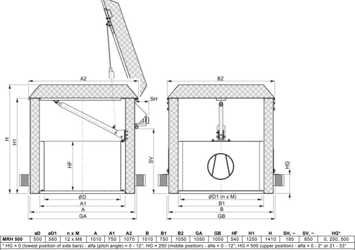
The side bars can be upon request ordered to meet specific roof pitch. More about side bar setting see instructions. MRH centreline deviation to vertical max. +/- 5°.
