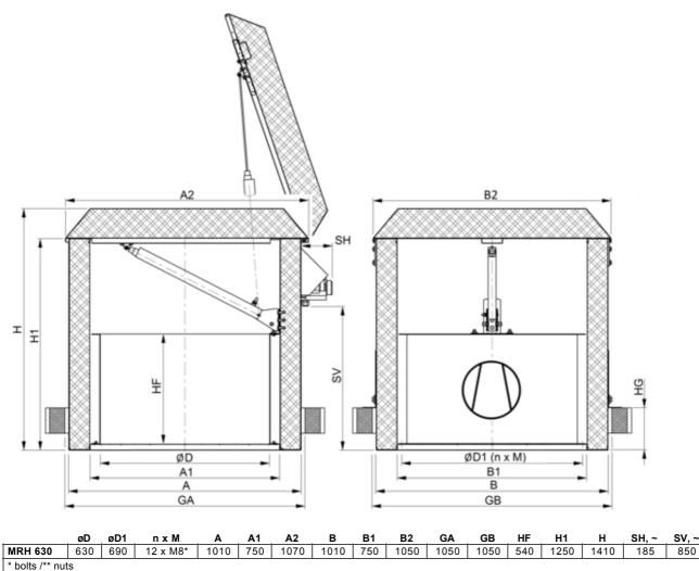
\*\*\*HG = 0 (lowest position of side bars) - alfa (pitch angle) =  $0 - 12^{\circ}$ ; HG = 250 (middle position) - alfa =  $0 - 12^{\circ}$ ; HG = 500 (upper position) - alfa =  $0 - 2^{\circ}$  or 21 - 33° The side bars can be upon request ordered to meet specific roof pitch. More about side bar setting see instructions. MRH centreline deviation to vertical max. +/- 5°.
