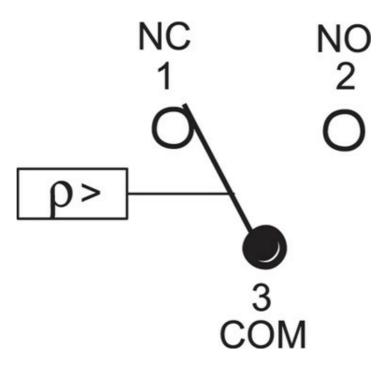
Switches from 1 to 2 when the pressure rises.
